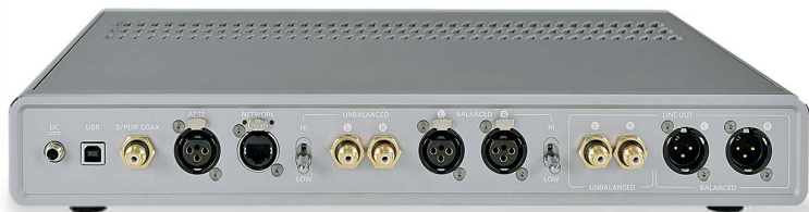
ABOVE: Powered via an outboard DC supply, the Aperio DAC/preamp includes USB, S/PDIF, AES3 and wired network ins alongside singled-ended (RCA) and balanced (XLR) analogue inputs (inc. high/low gain modes) and variable RCA/XLR analogue outs
